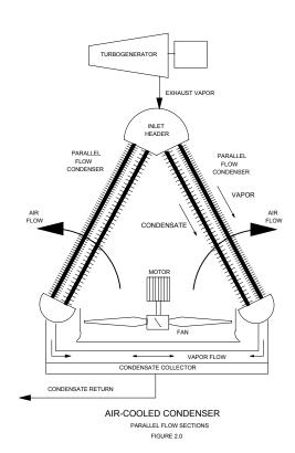
Fig 1. General View of Air-cooled Condenser
